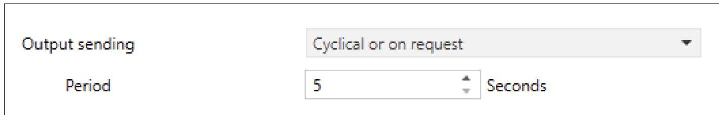
The "Output sending" parameter, when set to "Cyclical or on request", ensures that the output is transmitted either upon request or at regular intervals. The transmission frequency is defined in seconds using the "Period" parameter.
