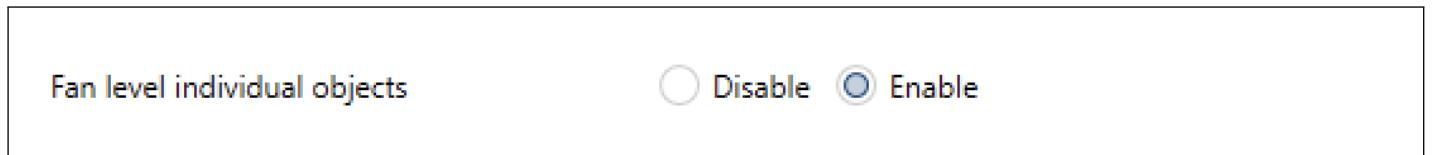
By activating the "Fan level Individual" Object, a separate object for each fan speed becomes visible, and each fan speed can be adjusted individually.
