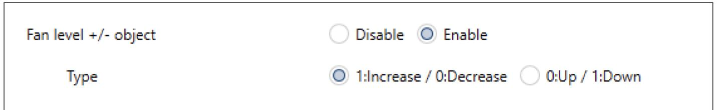
The Fan +/- Object parameter is used to switch between fan speeds. The direction of the transition between fan speeds is selected using the Type sub-parameter.
