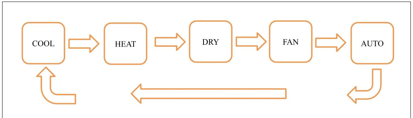
If the Type parameter is set to 0: Up / 1: Down, the mode transition sequence will be as follows:
