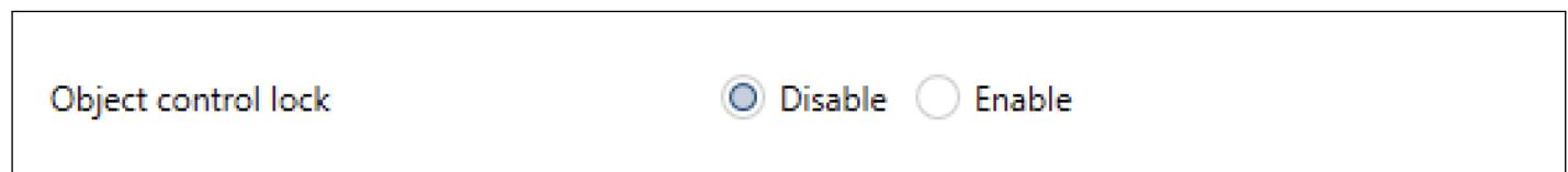
When the device lock is activated via the "**Object Control Lock**" object, the device becomes blocked and can no longer be controlled by any group object. Until the lock is deactivated, the device will not respond to any commands over the KNX bus. Even if the device receives a value during the locked state, it will retain its last status before the lock was applied once the lock is removed.
