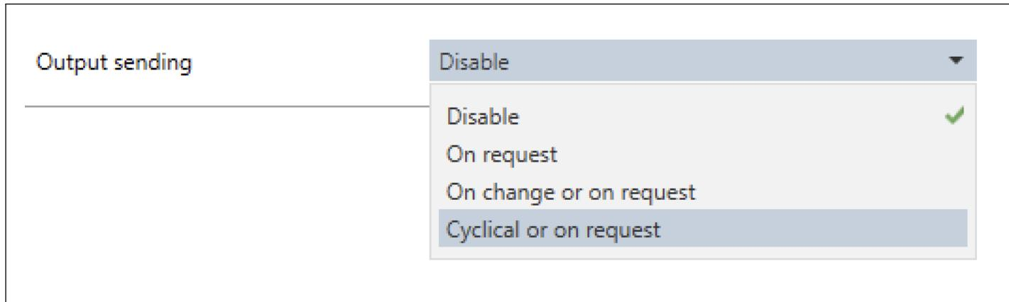
The "Output sending" parameter determines how the output is transmitted.
