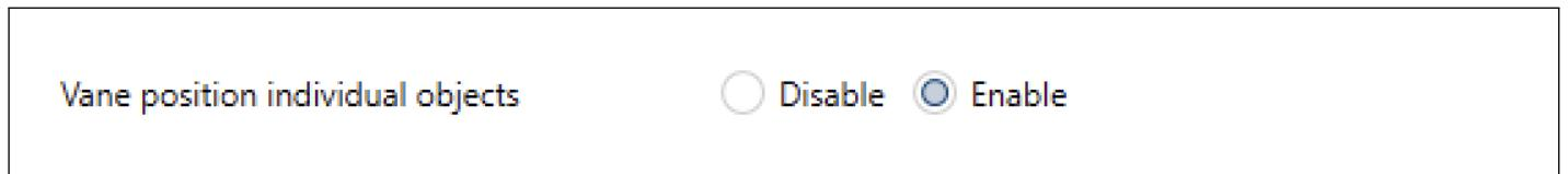
By activating the "Vane Position Individual Object," a separate object becomes visible for each vane position, allowing individual vane positions to be set separately.
